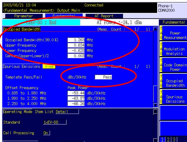
The evaluation result of spurious emission mask is comparable with the Template below.
